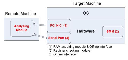
Fig. 1. The architecture of the memory forensics tool.
